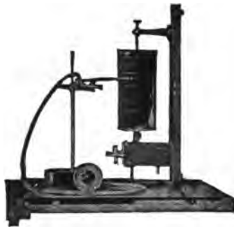
FIG. 129.—Apparatus for taking tracings of the abdominal aorta. The pulsations are conveyed by a cardiograph to a registering tambour.
