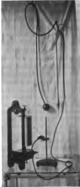
Fig. 42.—Apparatus for recording stomach-contractions incident to the action of transmitted energy. It consists of a stomach-tube to one end of which a rubber-balloon is fixed and to the other end a pump for inflating the balloon in the stomach. The pump and stomach-tube are connected with a piece of V-glass tubing. The stomach-contractions are transmitted to a tambour, the lever of which makes the record on a revolving cylinder.
