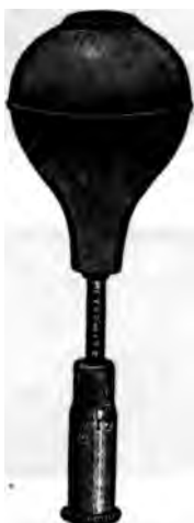
FIG. 4.—Galton whistle. This consists of a steel tube in which air is caused to vibrate. The note produced by it becomes higher as its length is diminished and ranges from 6,481 vibrations per second to the highest perceptible tone-limit.
