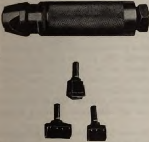
FIG. 50.—The author's pneumatic hammer with concussors.
