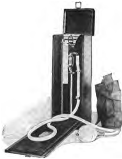
FIG. 11.—The Brown sphygmomanometer. The mercury cannot be lost and the cuff is 12 cm. in width, and 23 cm. in length.
