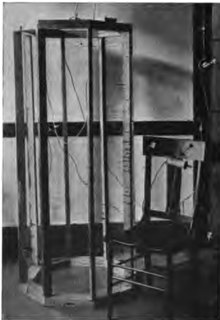
Fig. 40.—Helix and coil of wire (indicated by arrow) for demagnetization.
