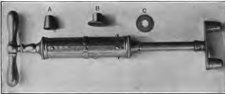
FIG. 1.—Spondylopressor with reflexometric attachment. A, attachment for use as an algesispondylometer; B, attachment for use as an algessimeter elsewhere in the body; C, attachment for gauging the vigor of the spinal and abdominal muscles.
