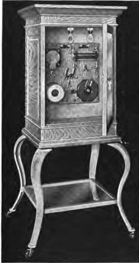
A FARADIC-GALVANIC ROLLER CABINET.
