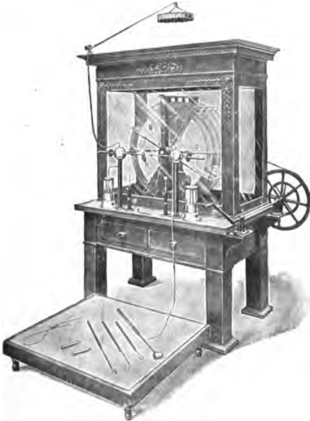
A MODERN TOEPLER-HOLTZ MACHINE.
