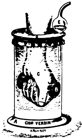
FIG. 3.—Hand-form plethysmograph. A, base; b, hand grip; c, hand; d, diaphragm; e, tube to recording apparatus.
