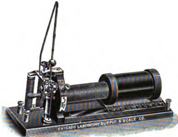
FIG. 15.—This figure shows an induction coil, which is used for applying the electrical stimulation to nerve trunks and other structures.
