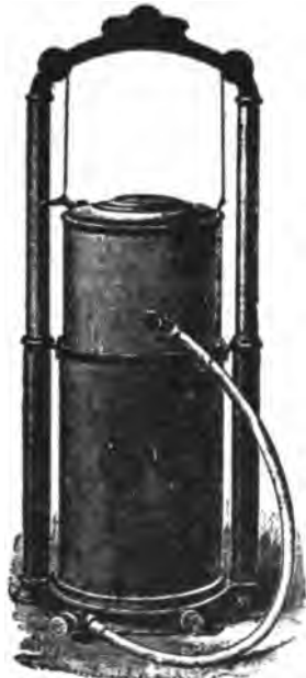
FIG. 16.—This figure shows a modern spirometer, which is used for studying respiratory capacities.
